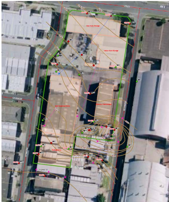
Figure 4-6: Groundwater flow as shown in GHD (2008)
