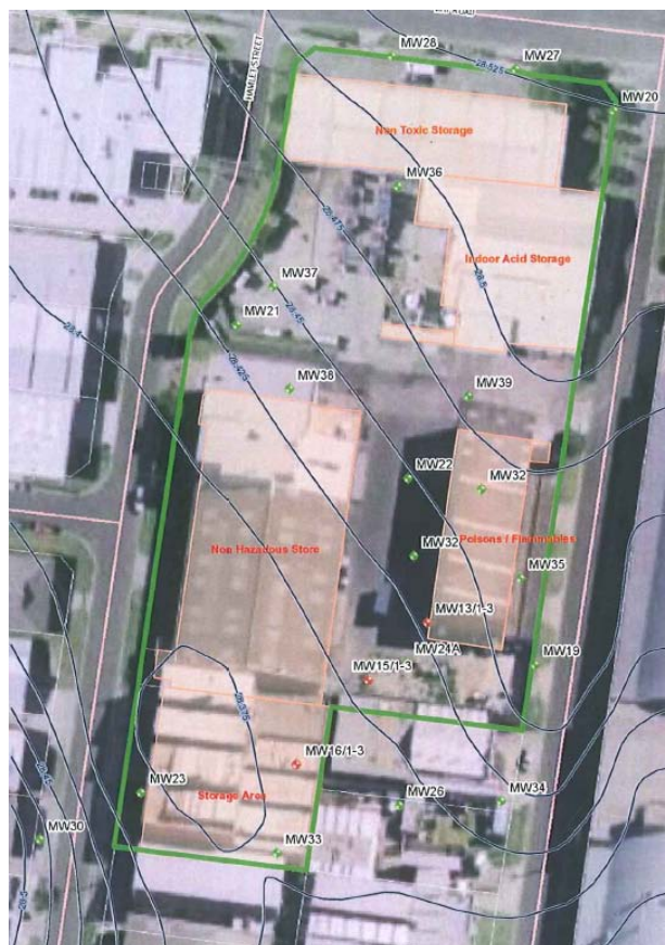
Figure 4-7: Groundwater flow as shown in GHD (2010)
